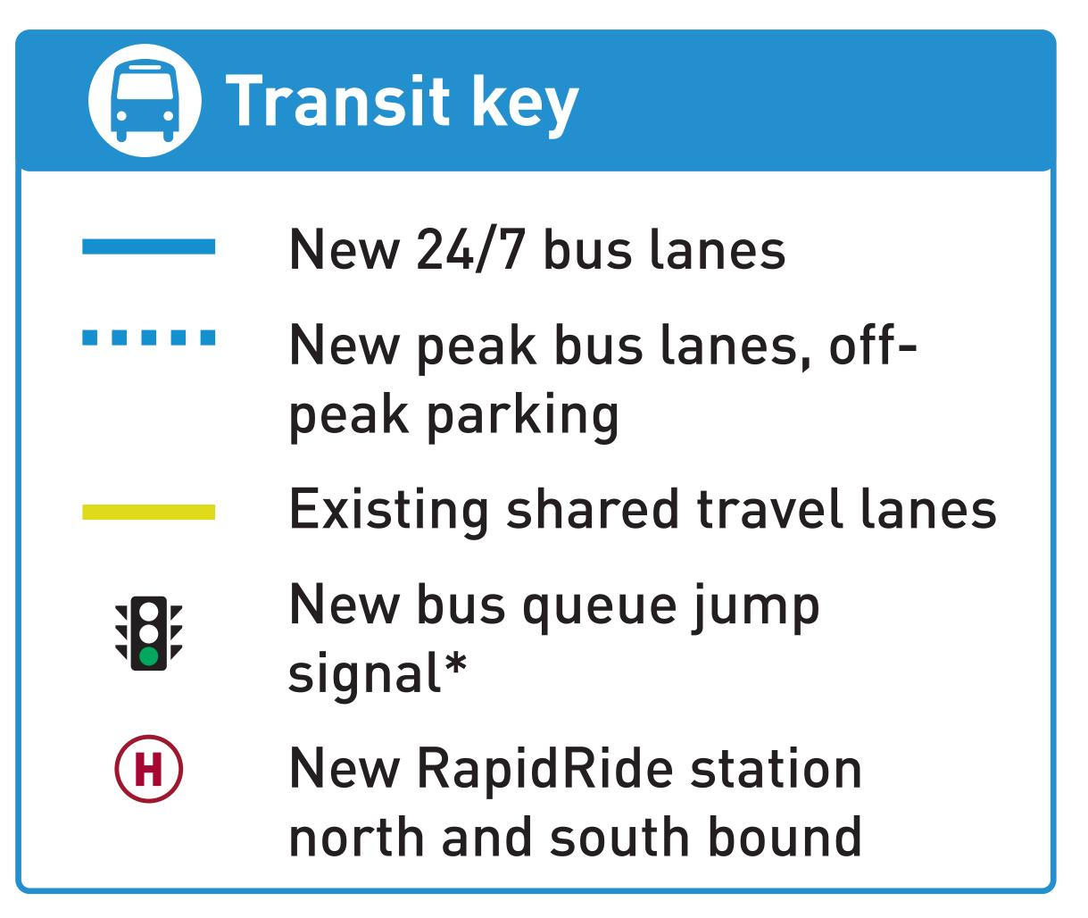
\*A bus queue jump is a traffic signal that gives buses in a separate bus lane an early green to get ahead of other vehicles at traffic lights to reduce delay and increase bus reliability.
